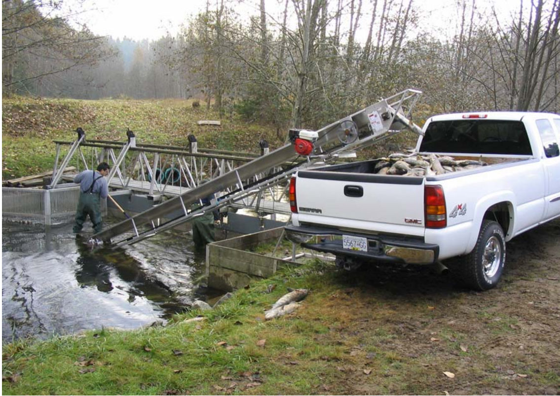
Loading a pick-up by conveyor belt at Little Qualicum spawning channel.
